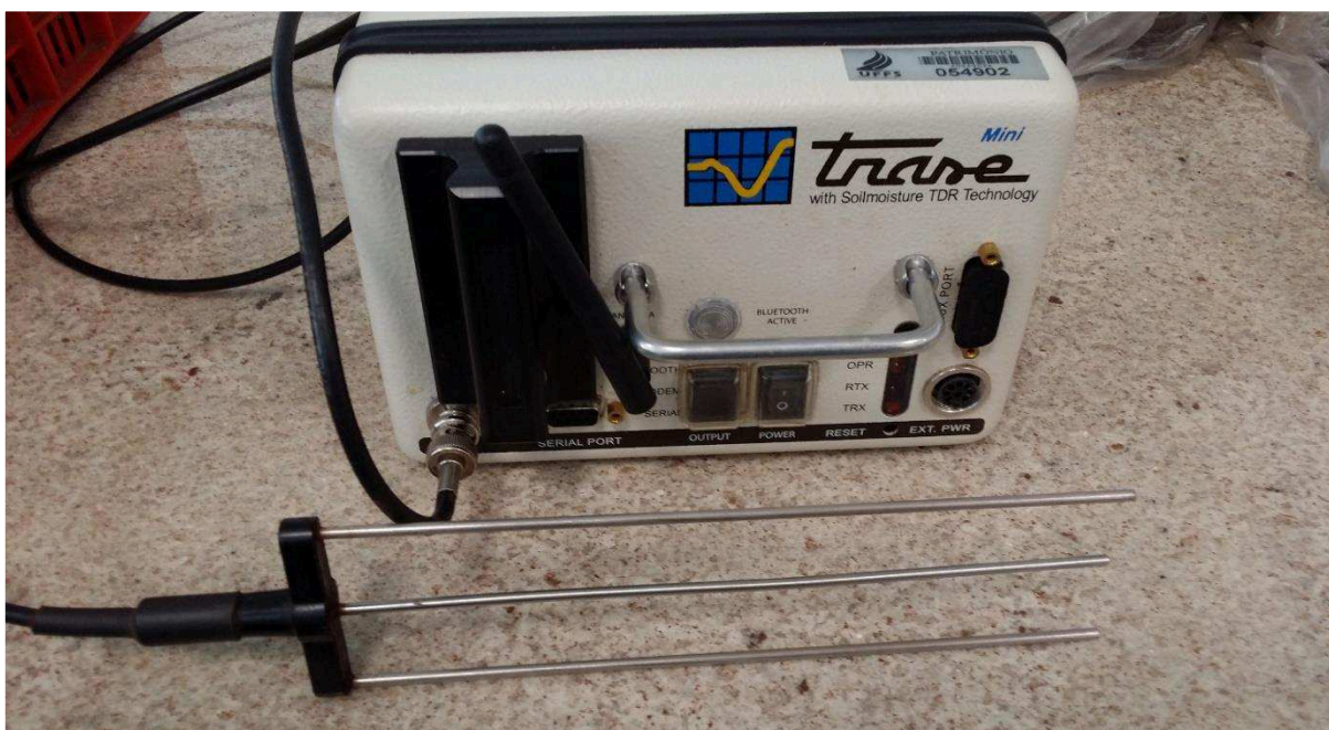
Figura 1 - TDR 6050X3K5B MiniTrase.
