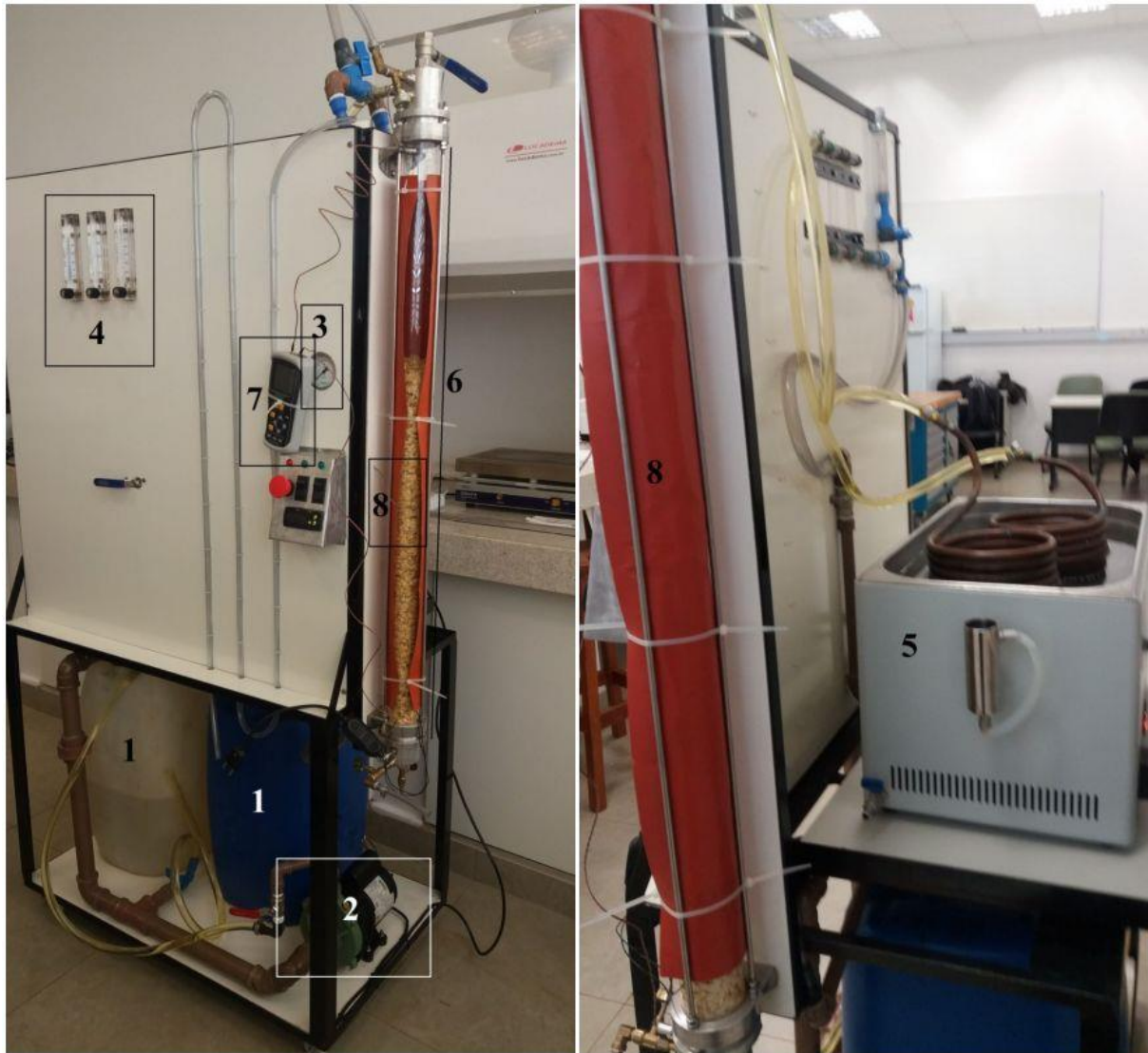
Figure 8. Experimental apparatus: isotherm column extraction.
